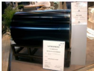
Coil coated selective absorber coating for solar thermal applications
